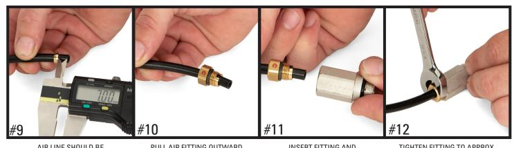
AIR LINE SHOULD BE APPROX. 6-8MM BELOW COLLET PULL AIR FITTING OUTWARD TO LOCK COLLET INSERT FITTING AND AIR LINE INTO VALVE
