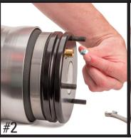
REMOVE THREADED PLUG AND DISGARD
