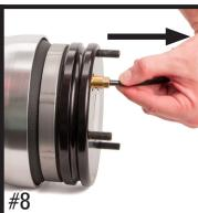
**GENTLY PULL ON AIR LINE TO** CONFIRM IT IS FULLY SECURED BY THE AIR LINE FITTING
