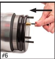
INSERT AIR LINE INTO THE AIR LINE FITTING UNTIL IT STOPS
