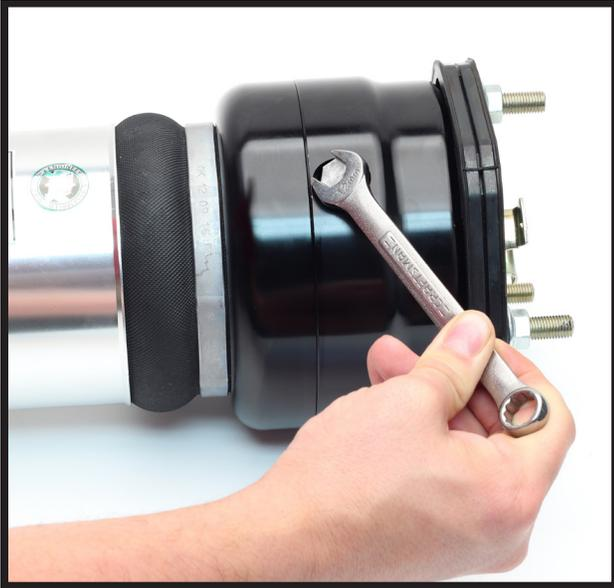
Install the air fitting, only until seated.
