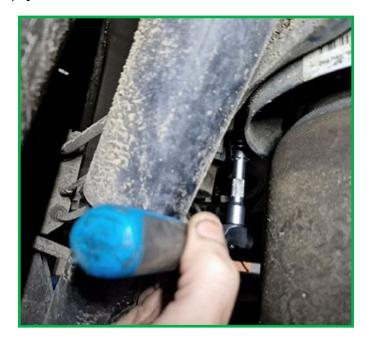
5. Carefully remove the air spring from the vehicle, to gain access to the air line. (Figures 5, 6)
