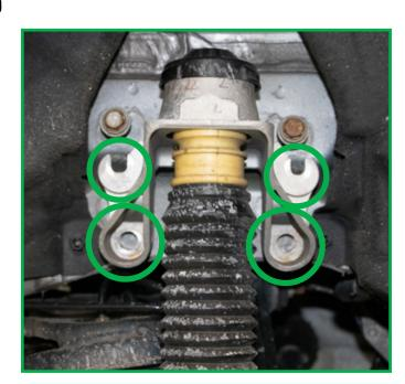
7. Remove the old shock from the vehicle. (Figure 7)
