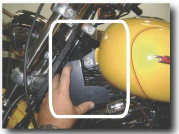
4. Place the compressor assembly over the front mounting bolt. Replace the mounting nut but leave loose for now.
