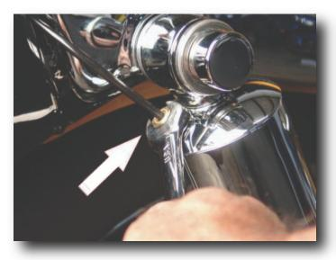
9. Connect each shock absorber to the distribution block with the 4mm line and VOSS<sup>®</sup> fittings supplied in the kit. Be careful to route the air line so that it does not kink. Instructions for assembly of the 4mm VOSS<sup>®</sup> fittings are enclosed in the kit. **NOTE:** Fittings seal with an o-ring, **DO NOT OVERTIGHTEN!**
