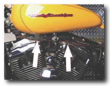
7. After connecting the 4mm air tubing to the compressor, route it beneath the left side of the fuel tank and along the frame toward the rear of the bike. Step #8 will cover connection to the distribution block using one of the 4mm VOSS<sup>®</sup> fittings supplied in the kit.
