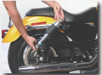
2. Install the ½ X 3" upper shock bolts and washers from the kit. Apply 2-3 drops of Loctite® 243 (blue) to the threads of each bolt. Torque all shock bolts to 45-50 ft lbs (61.1-67.9 Nm).
