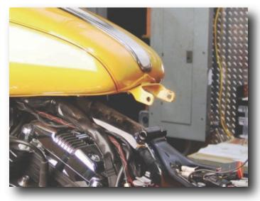
5. Remove the rear fuel tank mounting bolt and lift the tank slightly.
