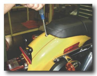
15. Reinstall the side cover and seat, make sure the seat tang is securely locked in the frame. Power up the system and use soapy water in a spray bottle to check for leaks.
