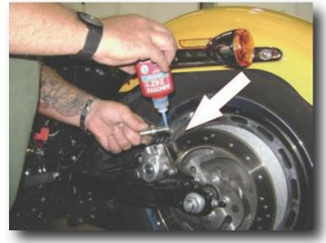
1. Install the new air suspension shocks one at a time. Start with the lower 3 1/4" bolts first. Then raise or lower the bike to line up the upper bolt holes.
