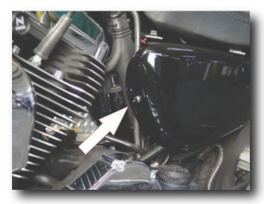
11. The preferred location for mounting the toggle switch is on the left side cover of the bike. Please refer to the system schematic on the back of the cover for a wiring diagram.
