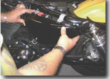
14. Reinstall the bike's side cover and the rear fuel tank mounting bolt. Torque the rear mounting bolt and the front bolt /nut previously loosened to 15-20 ft-lbs (20.4-27.1 Nm) Reconnect the battery, torque battery terminals to 60-96 in-lbs. (6.8-10.9 Nm).
