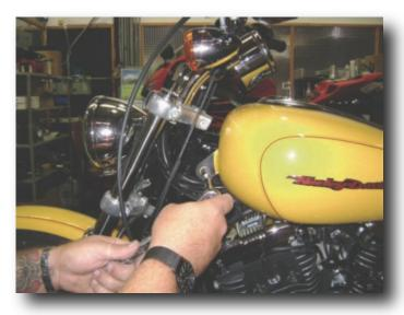
3. Locate and remove the nut located on the right front side of the gas tank.
