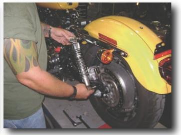
2. Carefully remove factory shock absorbers from the rear suspension.
