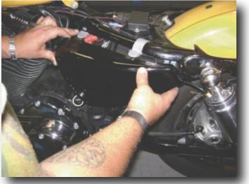
10. Remove the battery cover located on the left side of the bike. Disconnect the battery, negative cable (-) first.
