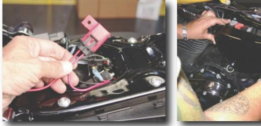
13. The preferred location for the fuse assembly is under the seat, near the battery. Connect the red wire with the ring terminal to 12V battery positive. Connect the other red wire from the fuse to the red wire of the switch.
