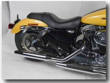
16. Make sure that there is adequate tire to rear fender clearance. Check both the center of the tire and the sides with the system in the lowered position, with zero air pressure.
