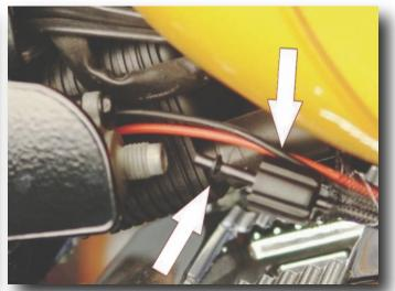
6. Locate the 4mm air line, the small o-ring and the retention cap that are supplied in the kit. Install the retention cap first, then the small o-ring onto the line. Insert the line into the compressor in the order shown above and tighten the cap.
