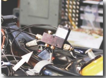
8. A preferred location for the solenoid vent valve/distribution block is under the seat.
