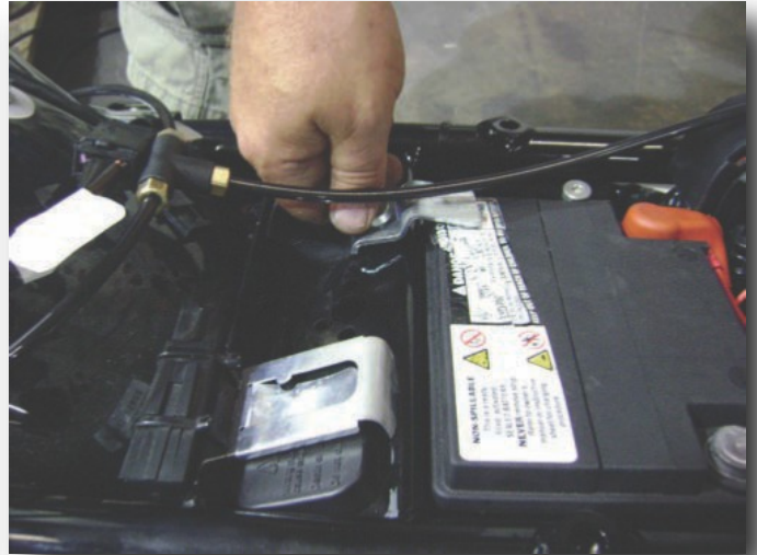
2. Disconnect and remove the battery. (Always remove the negative (-) cable first)
