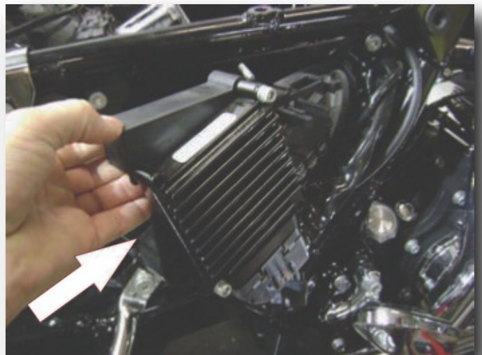
4. Using a thin wall 7/16" socket, remove the two nuts holding the control module located on the right side of the bike. Make sure you have complete access to the hole located under the battery box.
