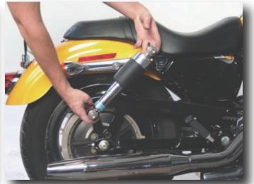
2. Install the new air suspension shocks one at a time. Start with the lower bolt holes first. Then raise or lower the bike to line up the upper bolt holes.
