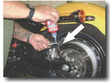
1. Remove the new ½ X 3" shock bolts and washers from the kit. Apply 2-3 drops of Loctite<sup>®</sup> 243 (blue) to the threads of each bolt. Torque all shock bolts to 45-50 ft lbs (61.1-67.9 Nm).
