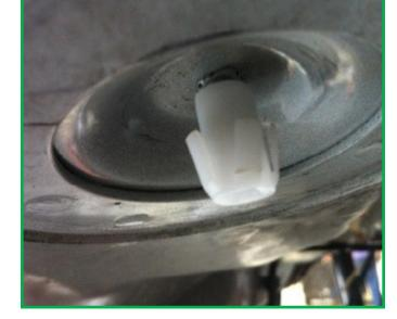
3. Install the upper spring seats onto the new clips. (Figures 42, 43)
