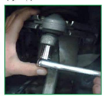
5. Separate the ball joint from the spindle assembly. (Figure 5)
