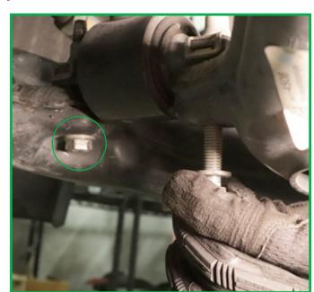
5. Remove the shock assembly from the vehicle. (Figure 8)
