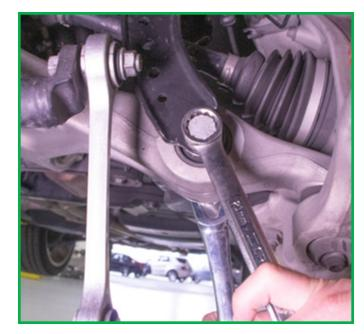
3. Reinstall the top sway bar end link bolt and nut and tighten to manufacturer's specifications. (Figures 26, 27)
