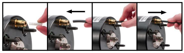
REMOVE AND DISPOSE OF THE SHIPPING PIN. INSERT AIR LINE INTO THE AIR LINE FITTING UNTIL IT STOPS. AIR LINE INSERTED.
