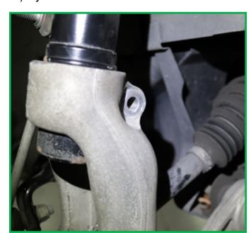
10. Use an appropriate tool to gently spread the clevis. Separate the strut from the strut mount. (Figure 14)
