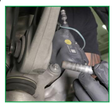
9. Locate and remove the struts three (3) top mount bolts. (Figures 11, 12, 13)
