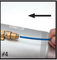
THREAD THE INCLUDED AIR LINE FITTING INTO THE VALVE
