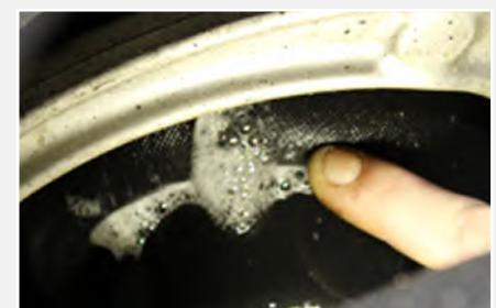
An air suspension leak is easy to find by spraying the air springs, struts and fittings with a soap and water solution. Bubbles will indicate where the leak or leaks are.
